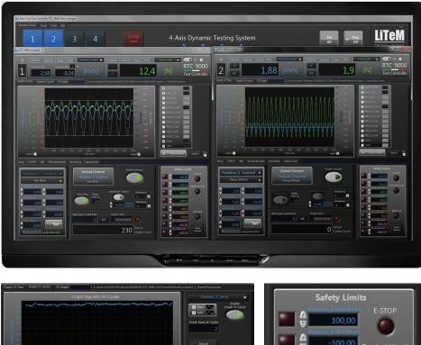
Display of all test parameters in a single clear and intuitive screen.
