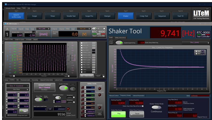
The frequencies can be set manually, automatically with the step function mode or automatically (frequency sweep mode).
