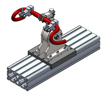
Clamps for static and fatigue tests - handlebar torsional security test ISO 4210-5: parte 4.5
