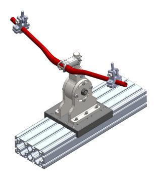
Clamps for static and fatigue tests - handlebar lateral bending test
