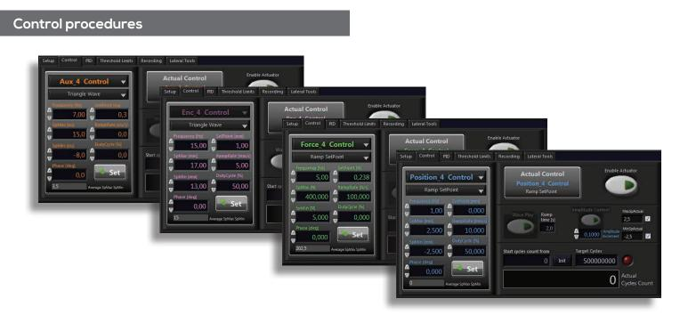
Possible control modes: Force, Displacement, Auxiliary and Encoder.
