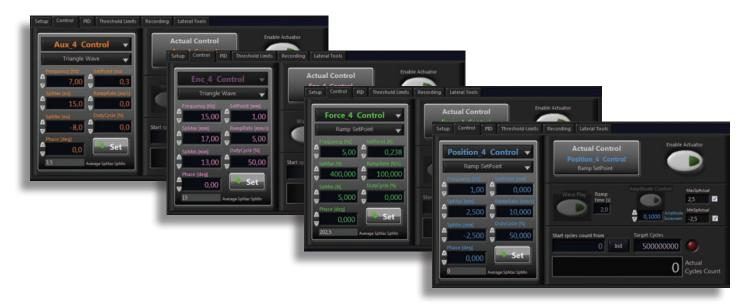
Possible control modes: Force, Displacement, Auxiliary and Encoder. Each mode can be set indifferently for each actuator even if they are operating simultaneously.
