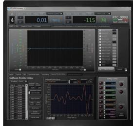
The SS 9000 software is designed to run static, semi-static and fatigue tests both with single-axis and multi-axis systems. Tests can be run either for:
