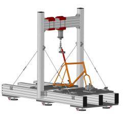
Frame: fatigue testing with vertical force
