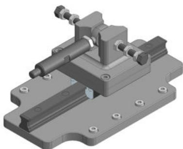
Allows the frame fork to be secured to the carriage positioned on the linear rail. The actuator rod which will generate the horizontal cyclical movement is connected to the carriage by means of the pin and the ball coupling.
